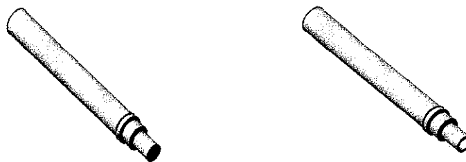
Figure 4.21: Drive Shaft (a) Initial design (b) Optimizing weight design
