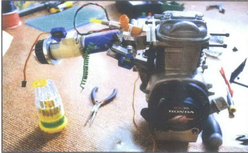
Figure 41: Speed reducer device on the engine
