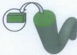
Figure 2.4: Fluid region of pipe flow discretized into finite set of control volumes
