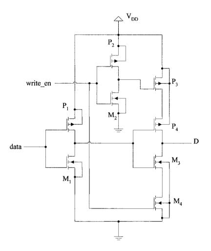
Figure 4 : Write Circuit for Input D
