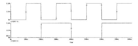
Figure 10 : Waveform of Input Signals for  $f_{CLK} = 10$  MHz
