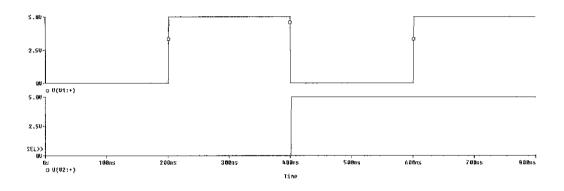
Figure 9 : Waveform of Input Signals for  $f_{CLK} = 5$  MHz
