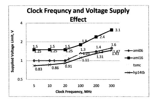
Figure 18 : Simulation using Different Process Technologies for Clock Frequency and Voltage Supply Effect
