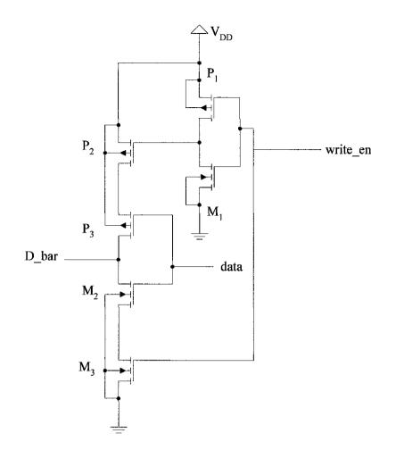
Figure 5 : Write Circuit for Input D bar
