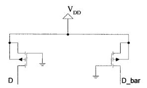
Figure 3 : Pull-up Circuit [5]
