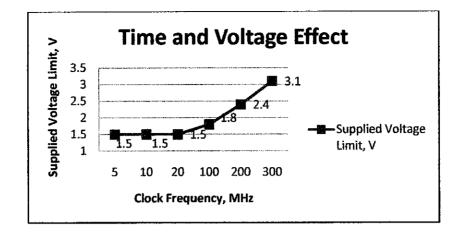
Figure 14 : Simulation Using ami16 Process Technology for Clock Frequency and Voltage Supply Effect
