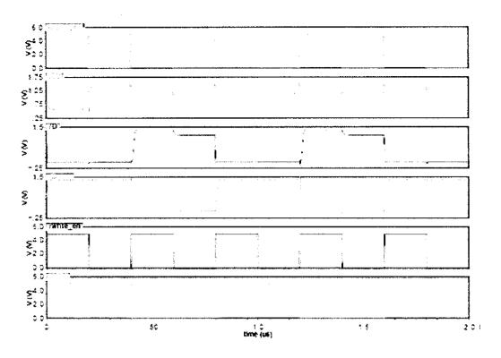
Figure 12 : Simulation for  $V_{DD} = 1.4$  V with  $f_{CLK} = 5$  MHz
