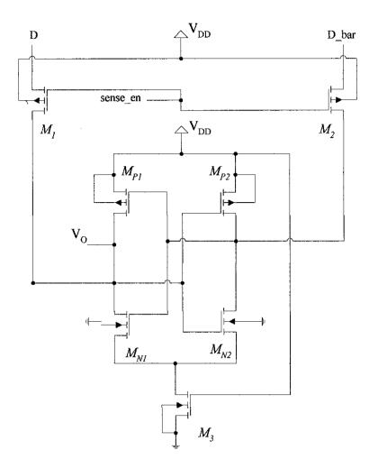
Figure 6 : Read Circuit Using Semi-latch Sense Amplifier
