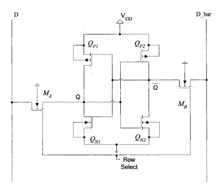
Figure 2 : 6T Cell Basic Memory Topology [11]
