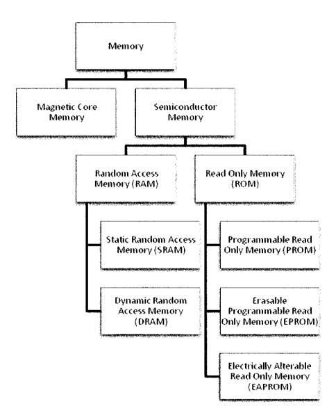
Figure 1 : Classification of memories in a digital computer [1]
