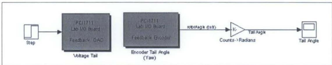
Figure 4.1 Tail rotor block diagram
