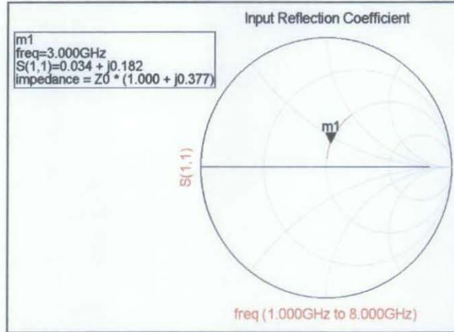
Figure 4.3: ADS Simulation Smith Chart for Single Series Inductor Circuit
