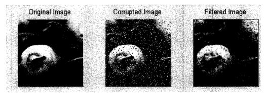
Figure 3 Effect of averaging filter on salt and pepper noise
