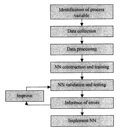
Figure 20 Methodology in developing the Neural Network (NN)
