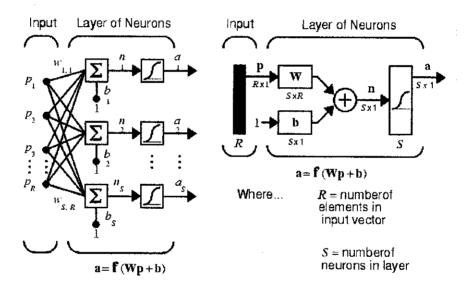
Figure 10 A single-layer networks (left) of S logsig neurons having R inputs and a layer diagram (right)
