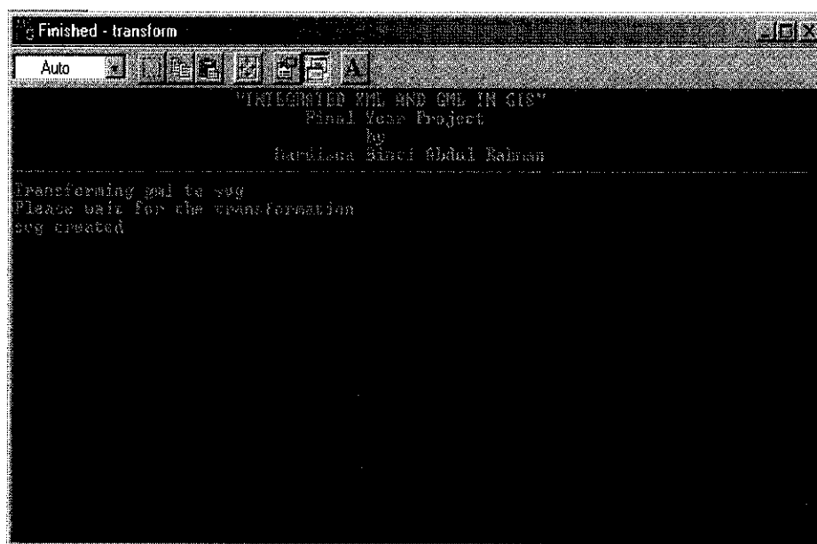
Figure 4.1: Transformation of GML to SVG Using Saxon
