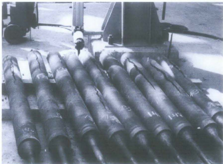
Fig.1: Photograph of nine failed tubes, as received [3]
