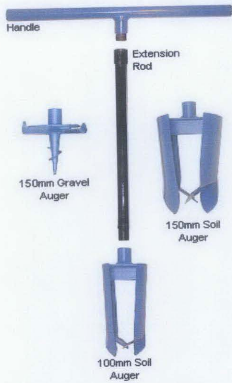
Figure 3.1: Diagram of Hand Auger
