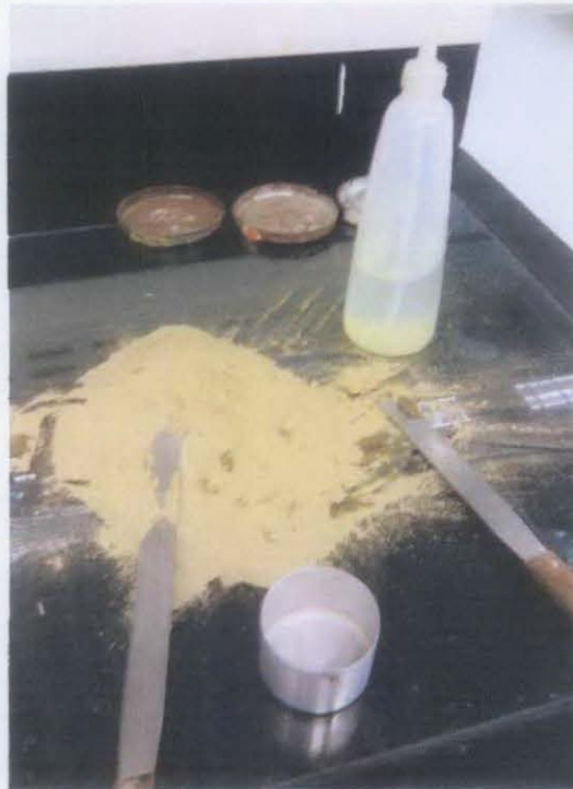
Figure B.3: Atterberg Limits (Plastic Limit Test)
