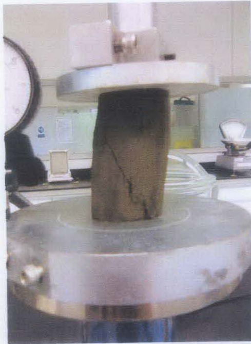
Figure B.1: Failure condition for marine clay-RHA at 7 days curing
