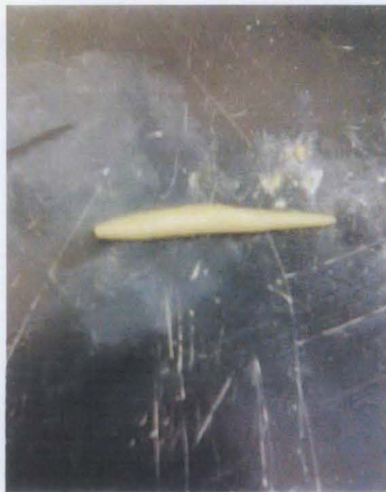
Figure B.4: Atterberg Limits (Plastic Limit Test)
