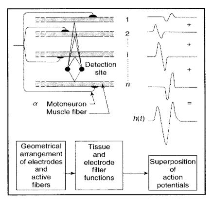
Figure 5: Schematic representation of the generation of the motor unit action potential
