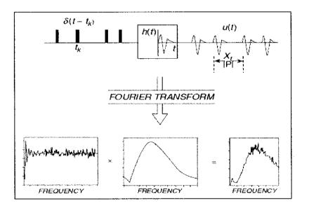
Figure 10: Model for a MUAPT in Fourier Transform modeling
