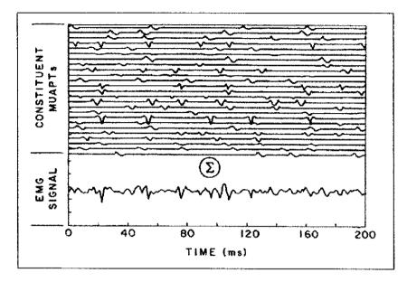
Figure 11: An EMG signal formed by adding or superimposing 25 mathematically generated MUAPTs.
