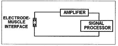
Figure 8: General circuit of the EMG acquisition system
