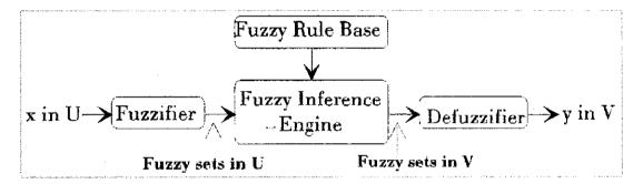
Figure 18: Basic configuration of fuzzy logic system with fuzzifier and defuzzifier
