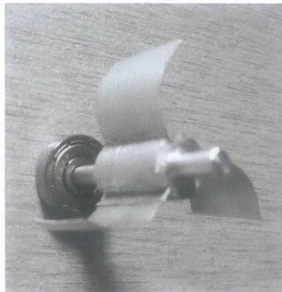
Figure 26: Three blades turbine after fabrication.
