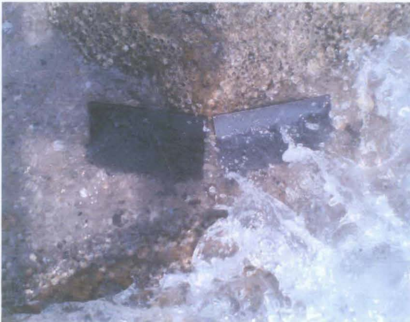
Figure 17: Two samples that being submerge in the seawater. Barnacle can be seen in the surface of the rock near the samples.
