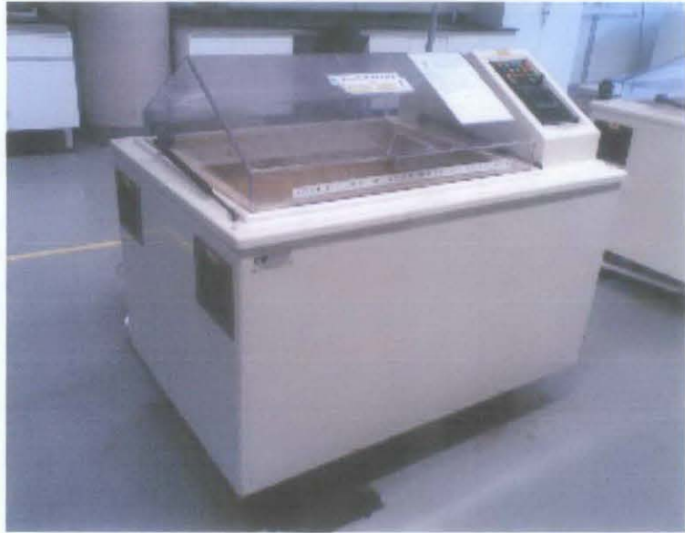
Figure 25: The exact same model of cyclic corrosion chamber at Block
