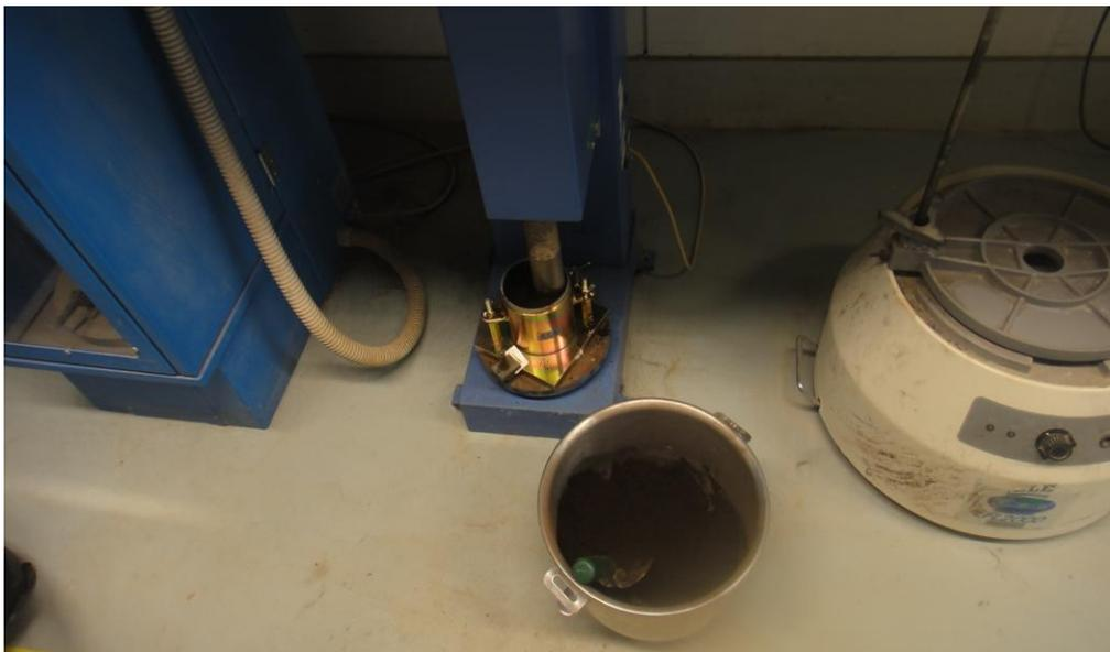
Figure 3.3.8: Standard proctor test
