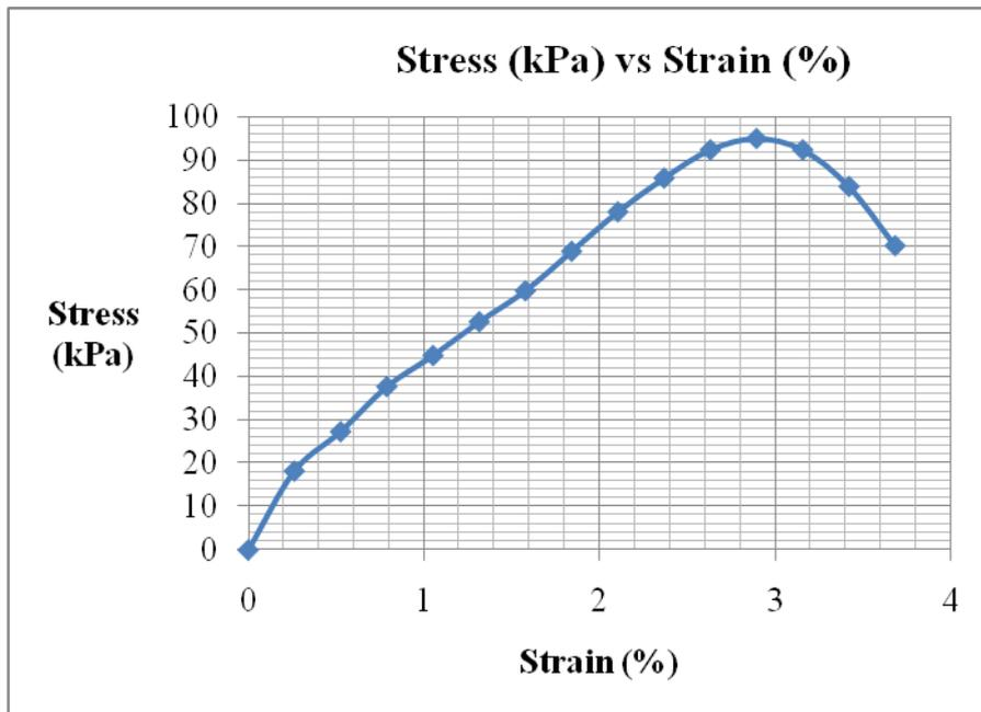
**Unconfined Compression Test Data (10% lime, cured for 0day)**
