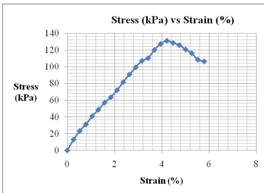
**Unconfined Compression Test Data (24% lime, cured for 14days)**
