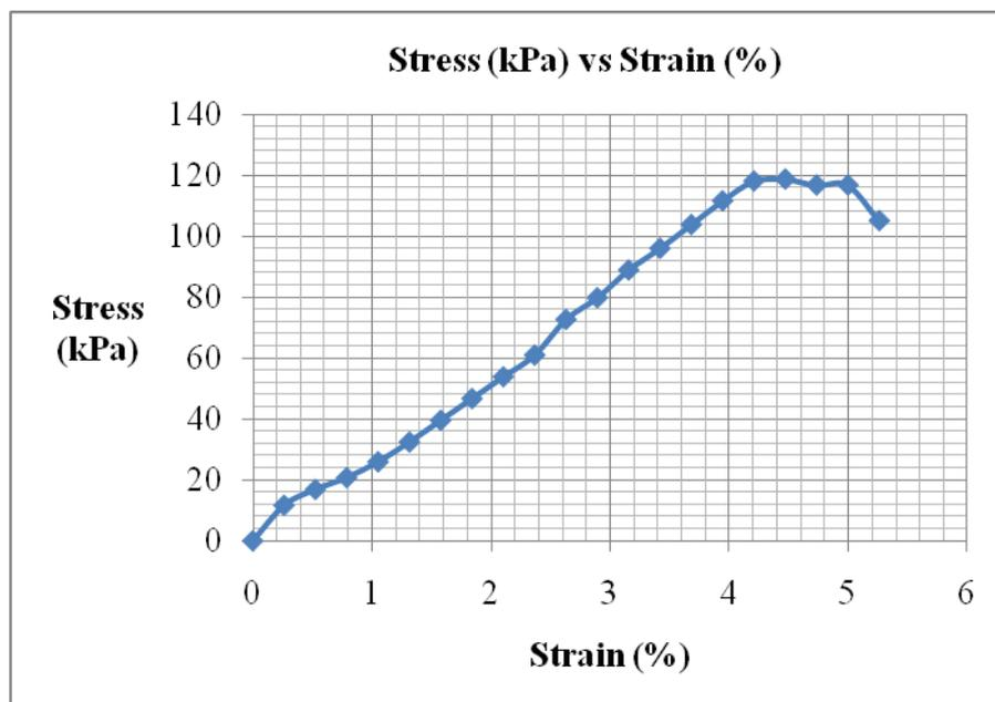
**Unconfined Compression Test Data (12% lime, cured for 14days)**
