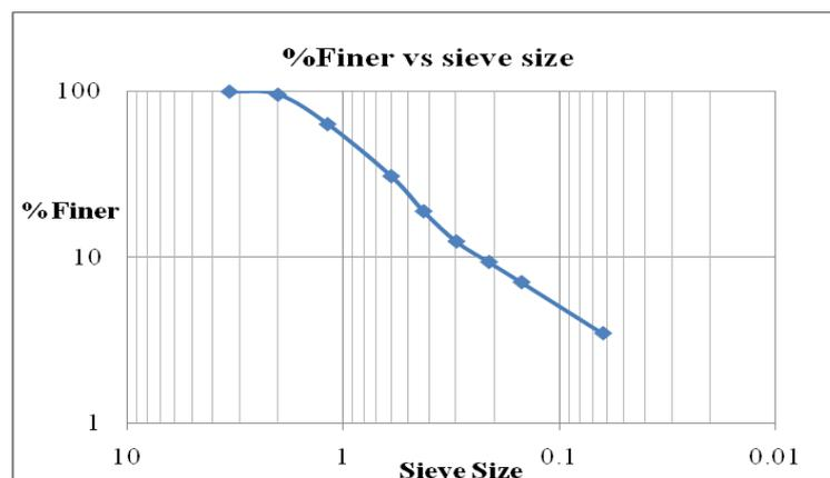
Figure 4.1.6: Particle size distribution (PSD) curve
