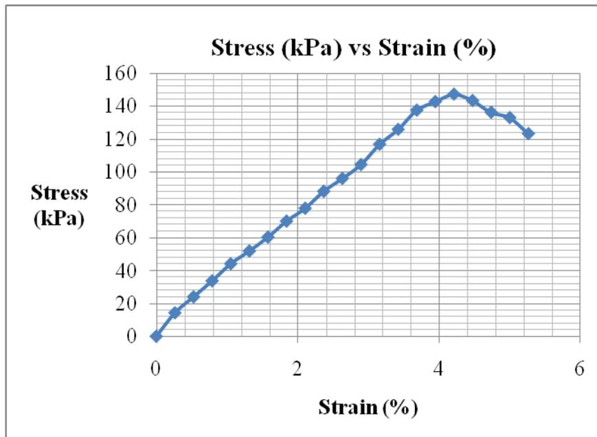
**Unconfined Compression Test Data (18% lime, cured for 14days)**
