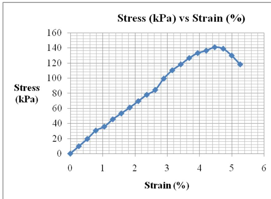
**Unconfined Compression Test Data (18% lime, cured for 7days)**
