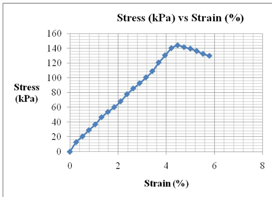
**Unconfined Compression Test Data (20% lime, cured for 14days)**
