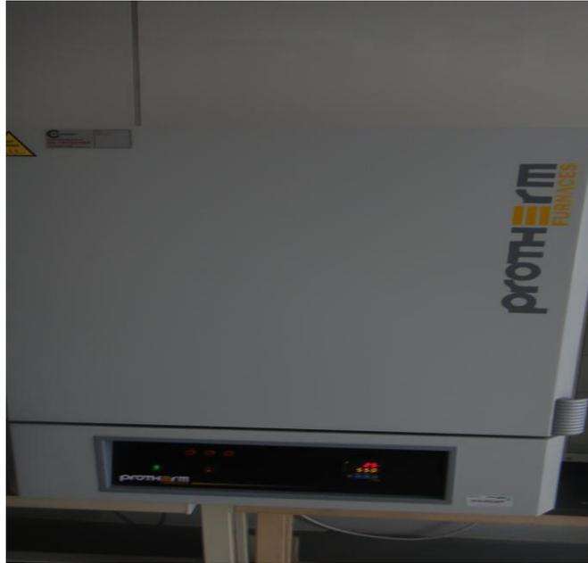
Figure 3.3.4: Muffle Furnace for determining peat organic content
