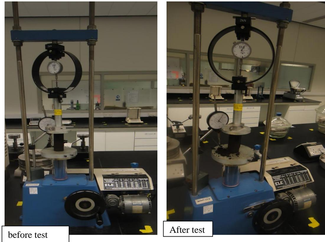
Figure 3.4.0: Unconfined compression test (UCT)
