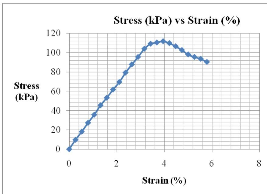
Unconfined Compression Test Data (**Samples cured for 0 & 7 days**)
