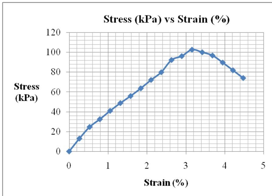
**Unconfined Compression Test Data (10% lime, cured for 7days)**
