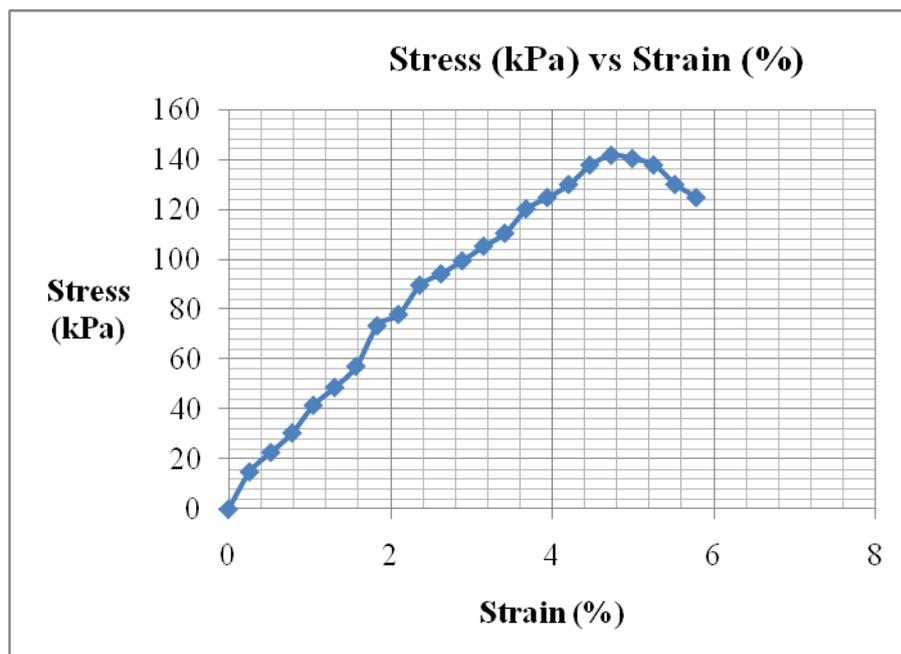
**Unconfined Compression Test Data (20% lime, cured for 7days)**
