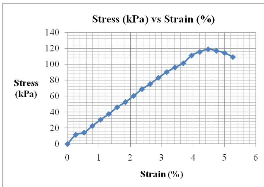
Unconfined Compression Test Data (14% lime, cured for 7days)
