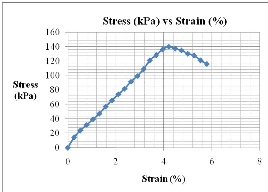
**Unconfined Compression Test Data (22% lime, cured for 14days)**
