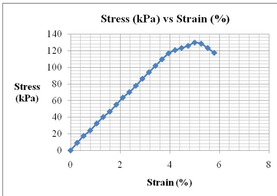
**Unconfined Compression Test Data (24% lime, cured for 7days)**
