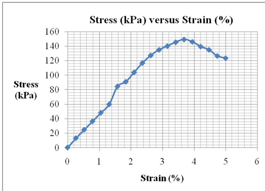
**Unconfined Compression Test Data (16% lime, cured for 14days)**
