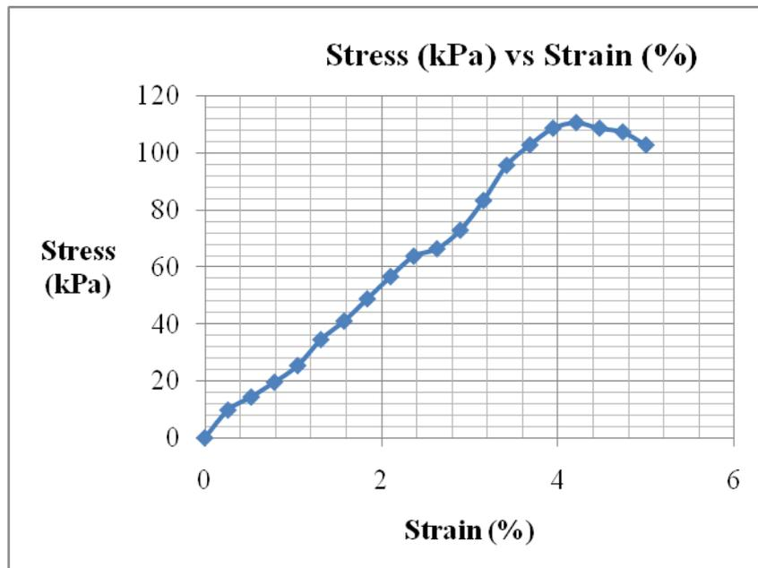
Unconfined Compression Test Data (12% lime, cured for 7days)
