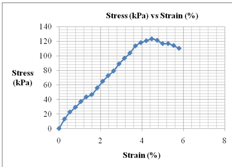
**Unconfined Compression Test Data (22% lime, cured for 7days)**
