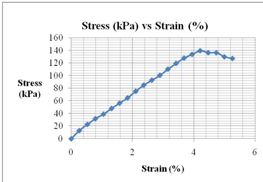
Unconfined Compression Test Data (14% lime, cured for 14days)
