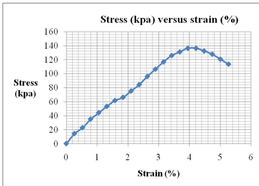
**Unconfined Compression Test Data(16% lime, cured for 7days)**
