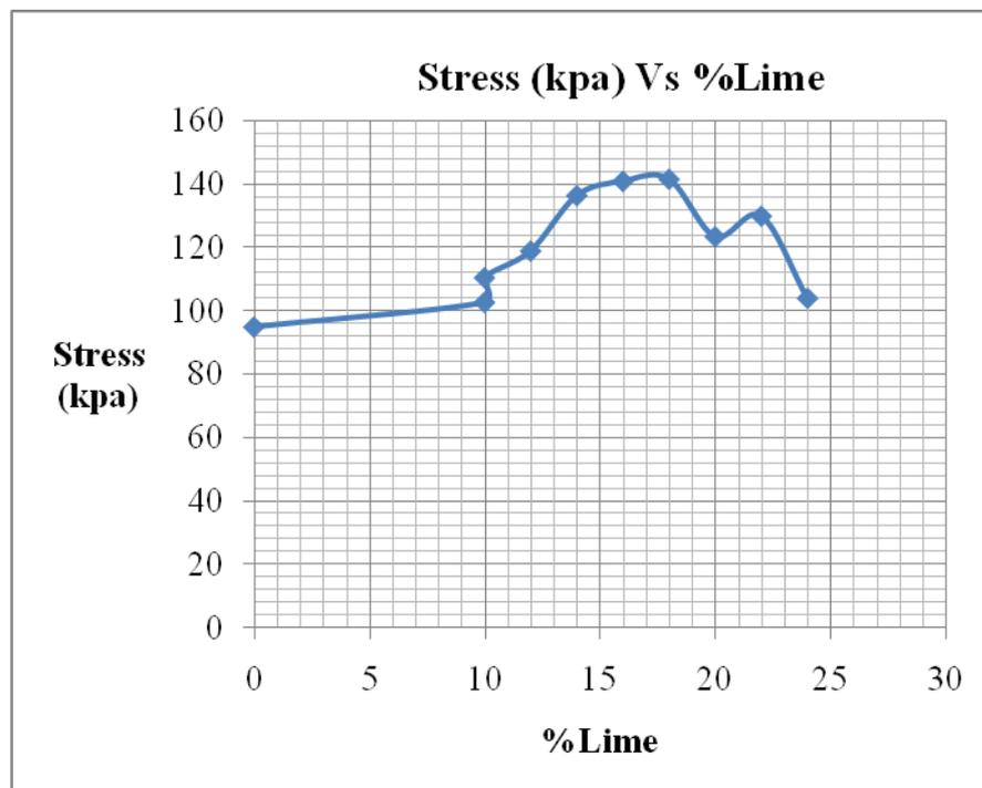
Unconfined compression test (UCT) data (**Samples cured for 0 & 14 days**)
