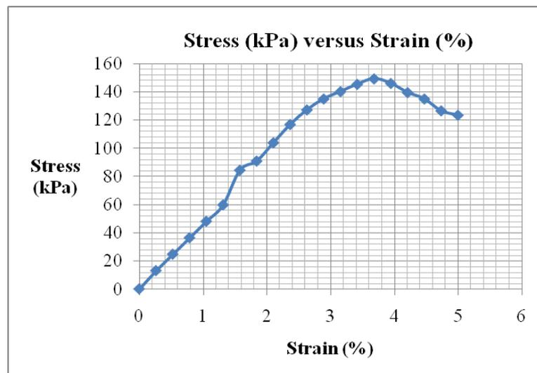
Figure 4.2.0: Stress (kpa) versus strain (%) of peat specimen mixed with 14% lime & cured for 14 days.
