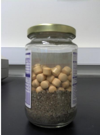
Figure 10: Glass container which will be used for ball milling process. One part is filled with jatropha sample, one part with ceramic balls and another part for ball milling space.
