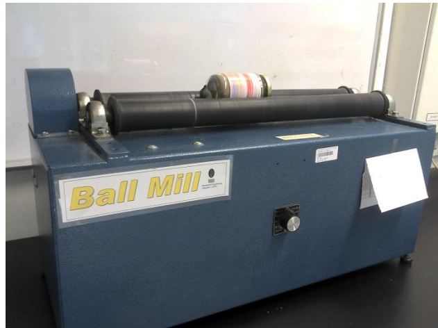
Figure 11: Ball milling in process. The speed was set to 100 rpm.
