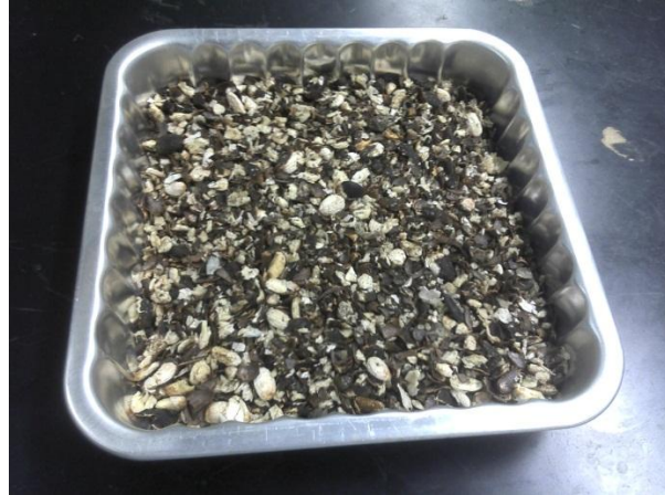
Figure 9: Jatropha seeds prepared in metal container before being put inside the oven for drying.
