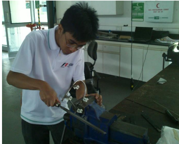
Figure 15: Smoothing of the frame's surface.
