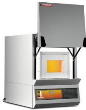
Figure 7: Furnace Test Machine used for char expansion
