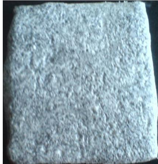
Figure 22: Coating applied for 10th formulation with fillers not grounded (2.0 gram of ATH and fumed silica, Sample 10)
