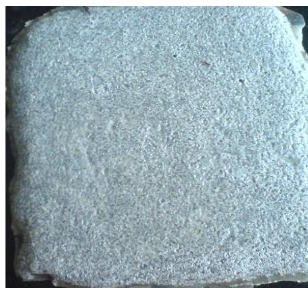
Figure 14: Coating applied for 2nd formulation with fillers grounded (0.5 grams of ATH and fumed silica, Sample 2)
