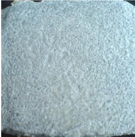
Figure 17: Coating applied for 5th formulation with fillers grounded (2.0 grams of ATH and fumed silica, Sample 5)
