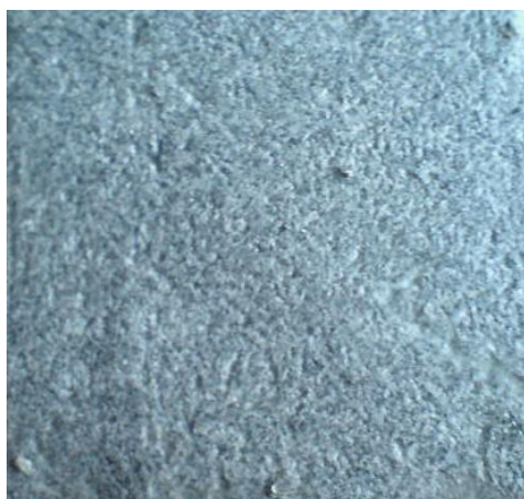
Figure 15: Coating applied for 3rd formulation with fillers grounded (1.0 gram of ATH and fumed silica, Sample 3)
