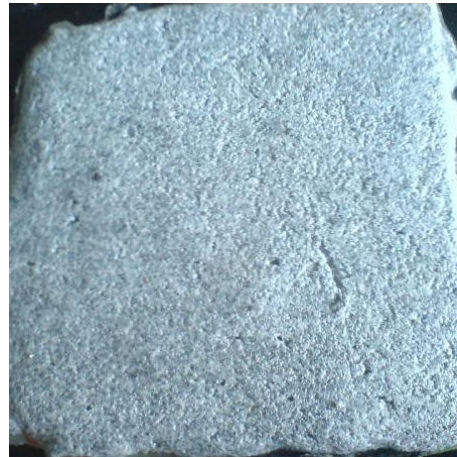
Figure 20: Coating applied for 8th formulation with fillers not grounded (1.0 gram of ATH and fumed silica, Sample 8)
