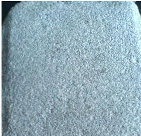
Figure 19: Coating applied for 7th formulation with fillers not grounded (0.5 gram of ATH and fumed silica, Sample 7)
