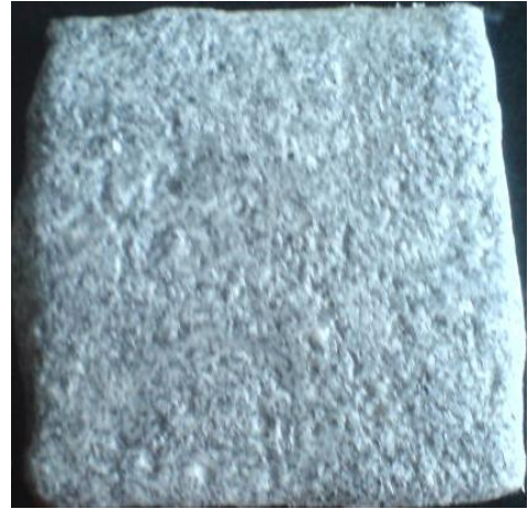
Figure 18: Coating applied for 6th formulation with fillers grounded (2.5 grams of ATH and fumed silica, Sample 6)
