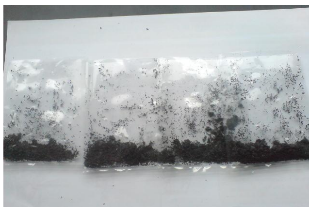
Figure 30: Char samples to be sent for XRD analysis
