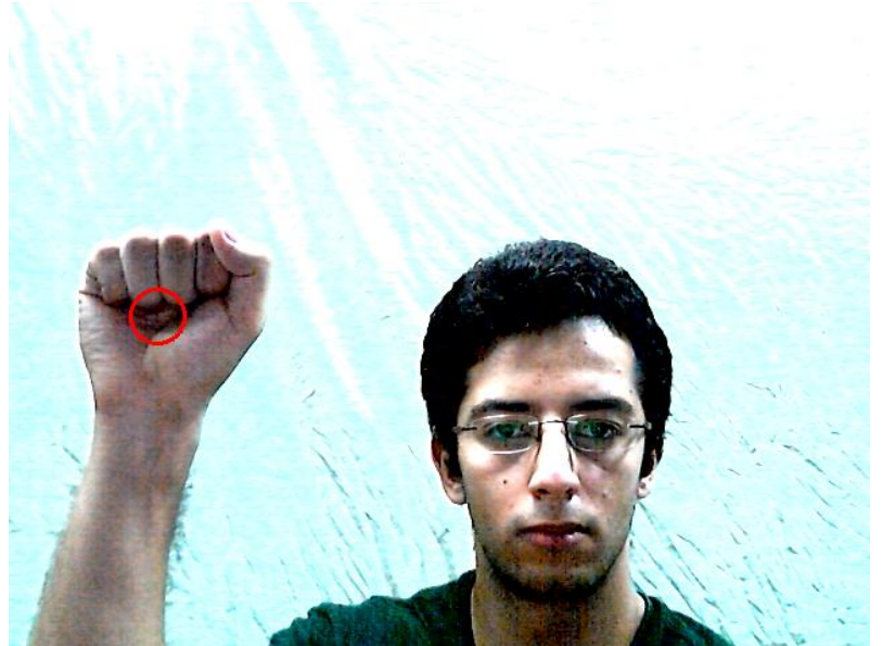
Figure 6 Closed hand gesture recognition using template matching, threshold=0.2, QVGA @30fps
