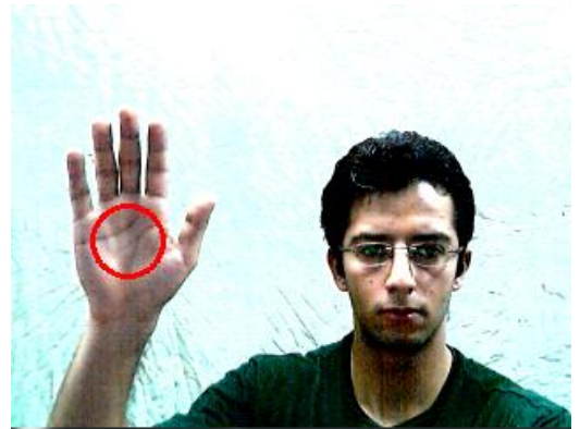
Figure 4 Open hand gesture recognition using template matching, threshold=0.2, QVGA @30fps
