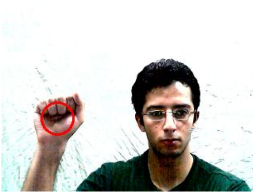
Figure 6 Closed hand gesture recognition using template matching, threshold=0.2, QVGA @30fps
