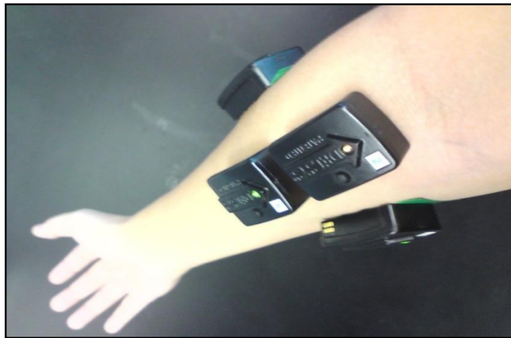
Figure 15: Placement of Delsys Trigno Wireless Sensor on subject's skin
