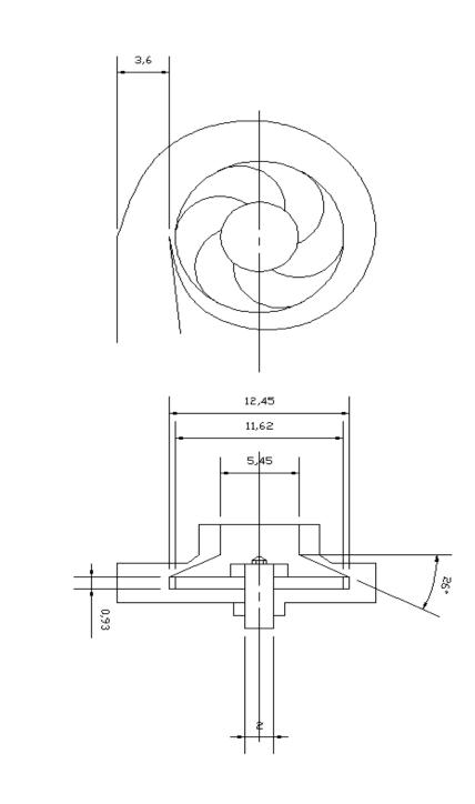
Figure 4.8: Assembly Drawing of the Centrifugal Pump
