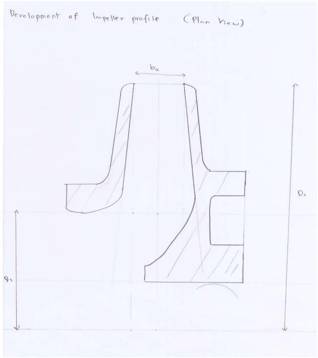
Figure 3: Impeller Layout (Plan View of Impeller Profile)
