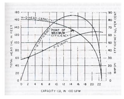
Figure 2.4: Pump Characteristic Curve [10]
