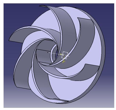
Figure 4.7: 3D Model of Impeller
