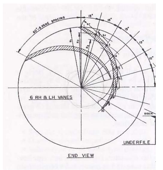
Figure 4: Impeller Layout Construction
