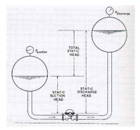
Figure 2.2: Static Head [10]
