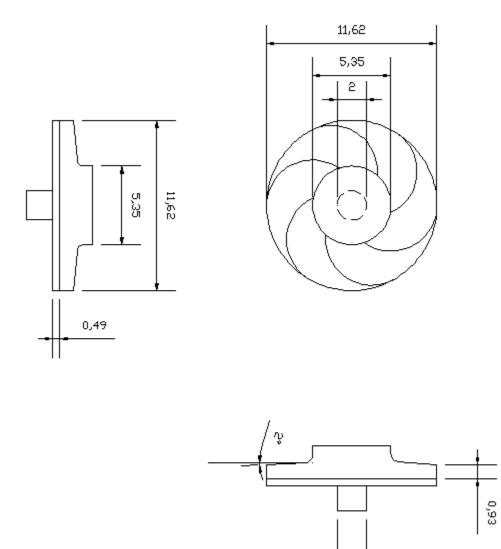
Figure 4.6: Technical Drawing of Impeller
