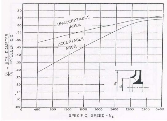
Figure 3.5: Impeller Eye Diameter/ Outside Diameter Ratio [6]
