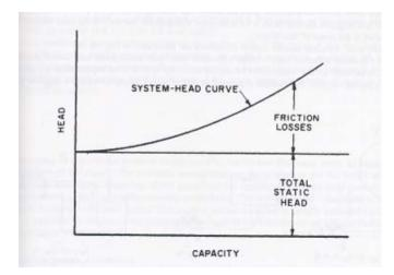
Figure 2.3: System Head Curve [10]
