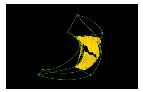
Figure 4.17: Pyramidal mesh element
