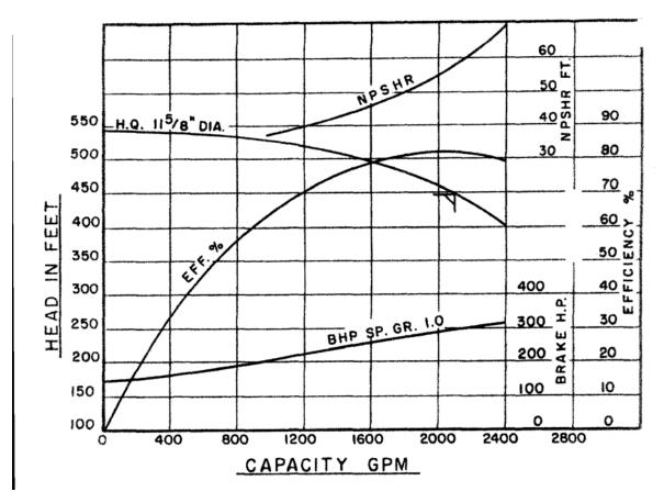
Figure 3.1: Required Performance of New Pump [6]
