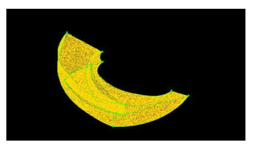
Figure 4.14: Meshed turbo volume for impeller blade
