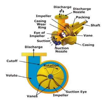
Figure 2.1: Important Parts of Centrifugal Pump [12]
