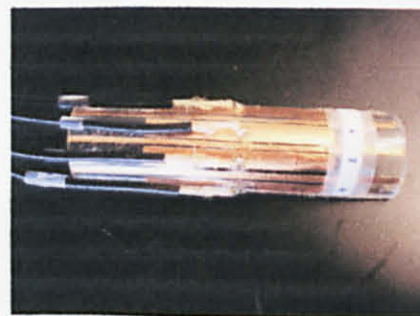
(b) Electrodes reside at the inner wall
