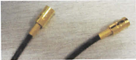
(b) RG-174 connected to SMB
