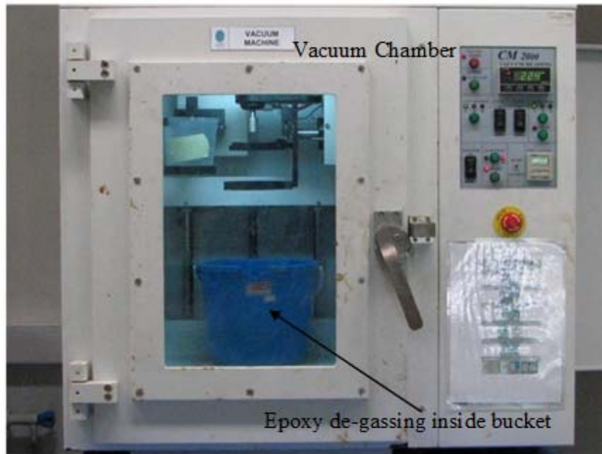
Figure 3.21 Epoxy being De-gassed inside the Vacuum Chamber
