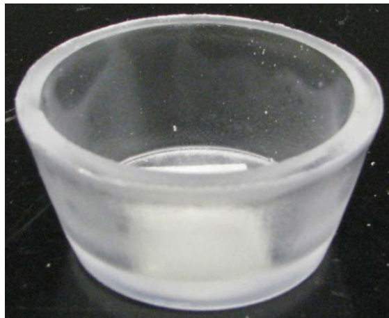
Figure 4.32 Part produced with Injection Moulding
