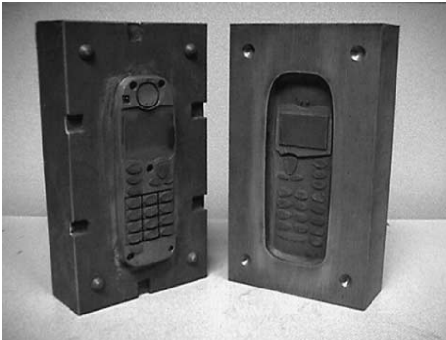
Figure 2.7 Injection Moulding core and cavity produced with RT [31]
