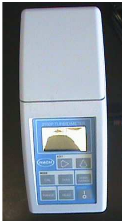
Figure C.4 The Hach 2100P portable Turbidimeter
