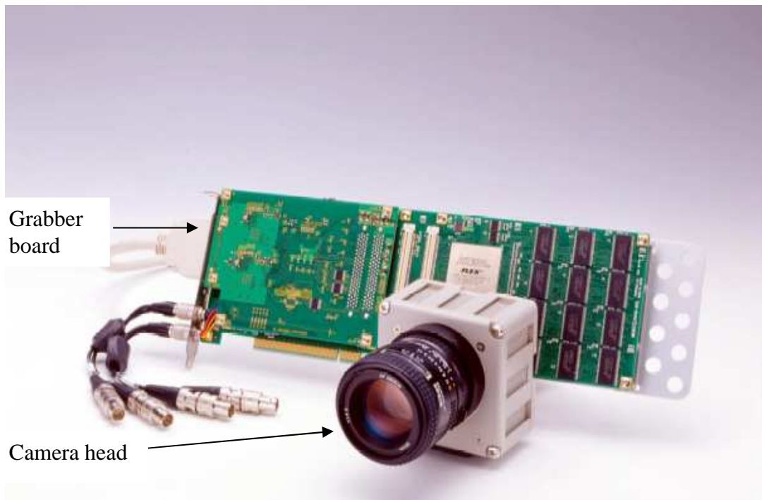
Figure C.2 The Fastcam-x1280pci camera head [87].
