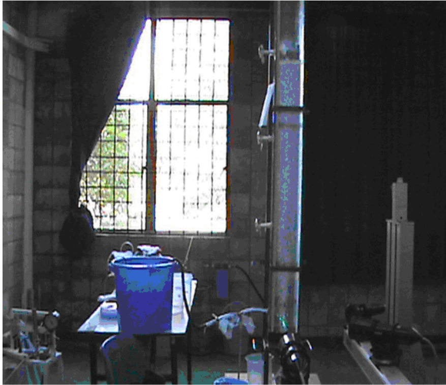
Figure A.2: The experimental set-up water column (120 mm W x 120 mm L x 2 m H).
