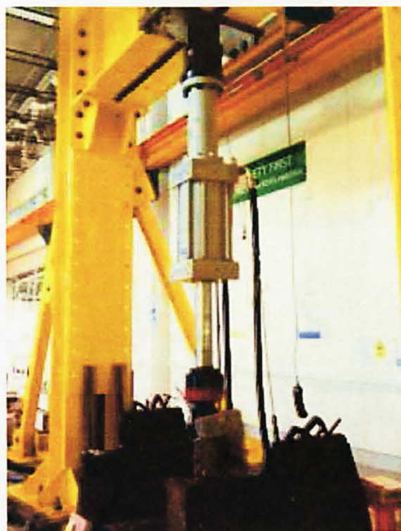
Figure 7: Self Straining Loading Frame
