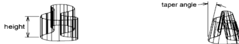
(a) Extrude with a height and 0 angle (b) Extrude with negative angle – taper in
