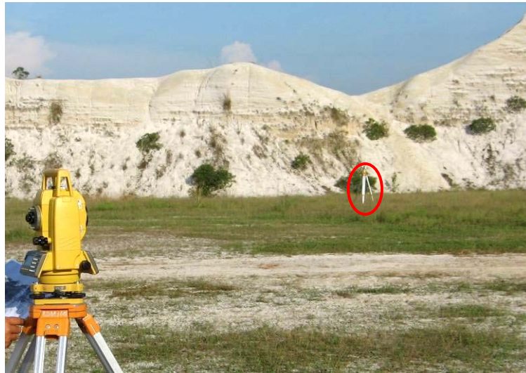
Figure 3.11. Position of the TS (on occupied point) and the standard single prism (on back-sight point) in the field measurement process
