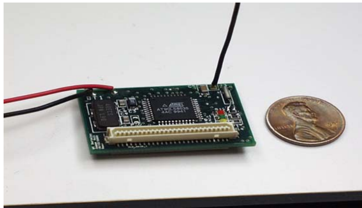
Figure 2-1: University California at Berkeley (UCB) Rene Motes used by the Laboratory of Experimental Computer Sciences (LECS).
