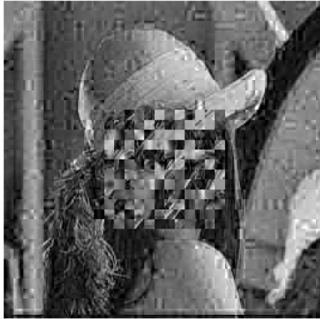
Figure 6.5: 256×256 center selected Lena Image 5 th , 4 th and 3 rd AC coefficient scrambled (PSNR = 17.88, SSIM = 0.5167, MS-SSIM = 0.6089, VIF = 0.1472, VIFP = 0.2097, VSNR = 8.19, UQI = 0.4298).
