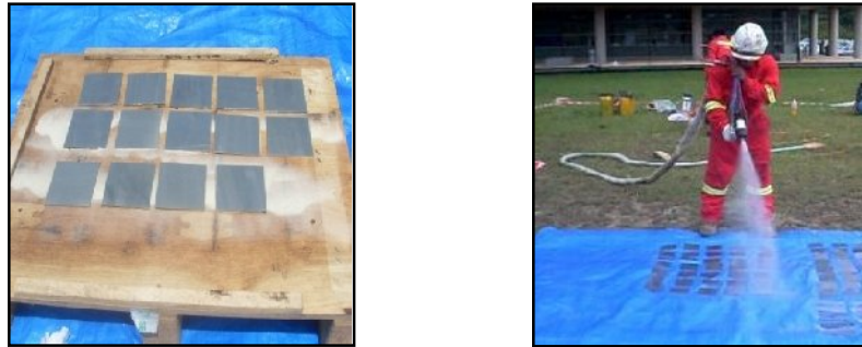
Figure 3.4: Coating process by Dyna Segmen (M) Sdn Bhd
