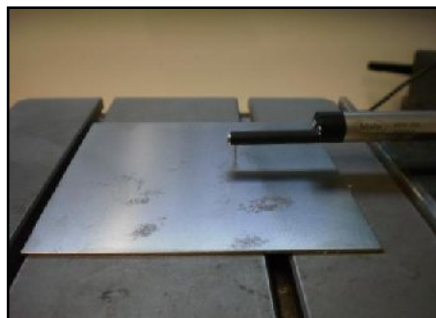
Figure 3.3: Measure the surface roughness; Ra using the surface profiler machine (Before/after Coating)
