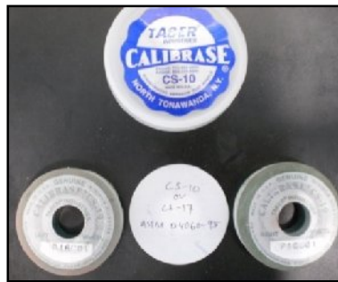
Figure 3.6: Calibrase CS-10 as per ASTM D4060-95
