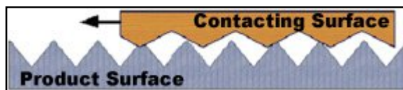
Figure 2.3: Process of the Wear Abrasion Resistance
