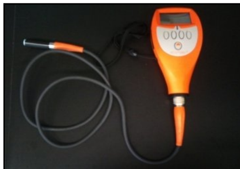
Figure 3.7: Dry Coating Thickness
