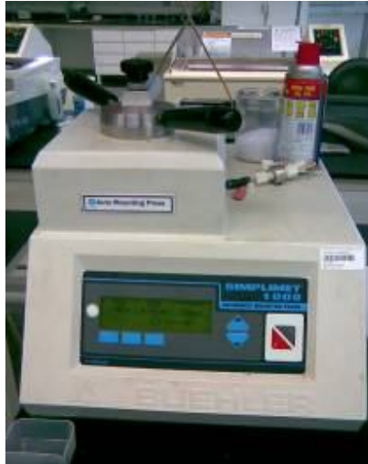
Figure 4.6: Equipment used for mounting
