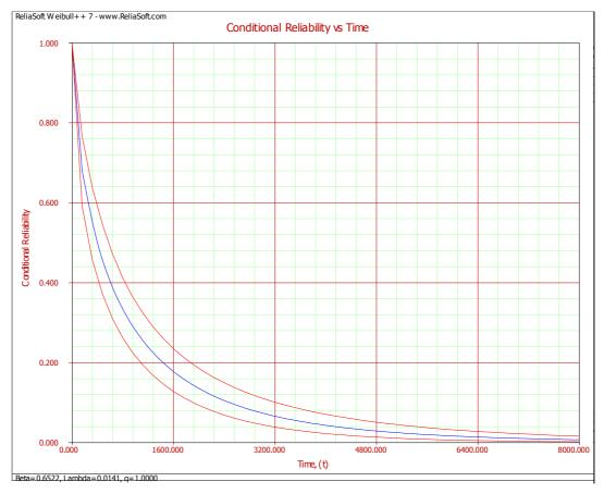
Figure 4.13: Conditional Reliability versus Time Graph for 2000 Operation Days
