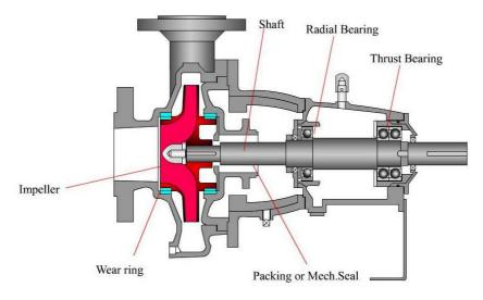
Figure 2.3: Centrifugal Pump Components [17]
