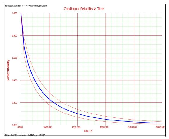
Figure 4.7: Conditional Reliability versus Time Graph for the Pumps
