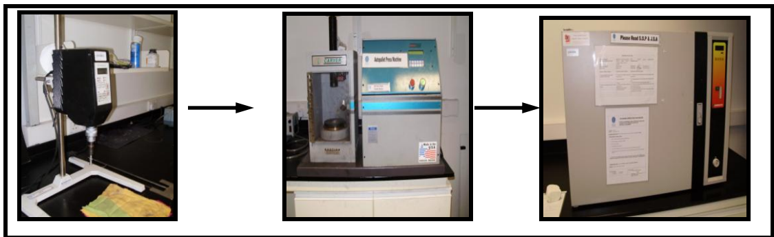
Figure 3.1: Process flow of manufacture bonded NdFeB starting with stirrer (picture 1), Auto Pallet Machine (picture 2) and oven (picture 3)
