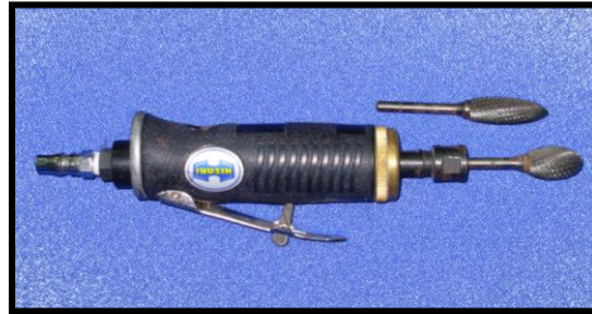
Figure 1.1: Micro grinder machine with pineapple bit
