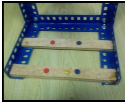
Figure 4.11: The location of 4 bonded NdFeB magnets on steel attachment
