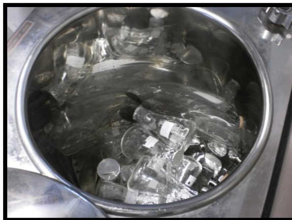
Figure 20: Media for algae growth is being sterilize in an auto clave machine at 121 0 C for 15 minutes
