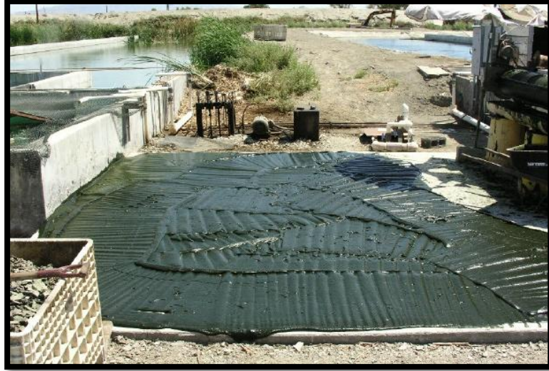
Figure 25 : Example of industry belts harvest and drying process of algae(Brune et al, 2010)
