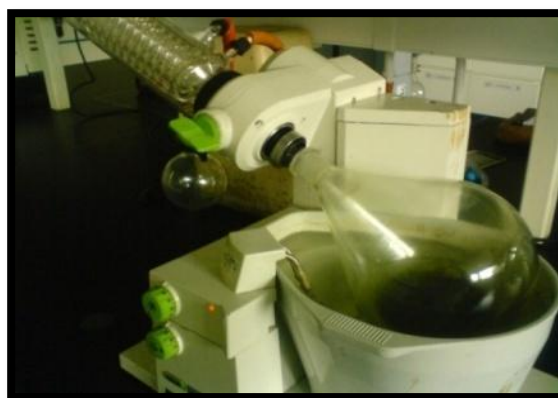
Figure 27 : Rotary Evaporator evaporates chloroform
