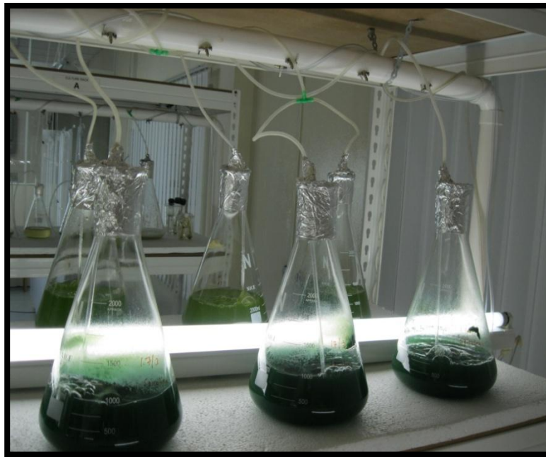
Figure 22 : Microalgae with agitation(bubling agitation)
