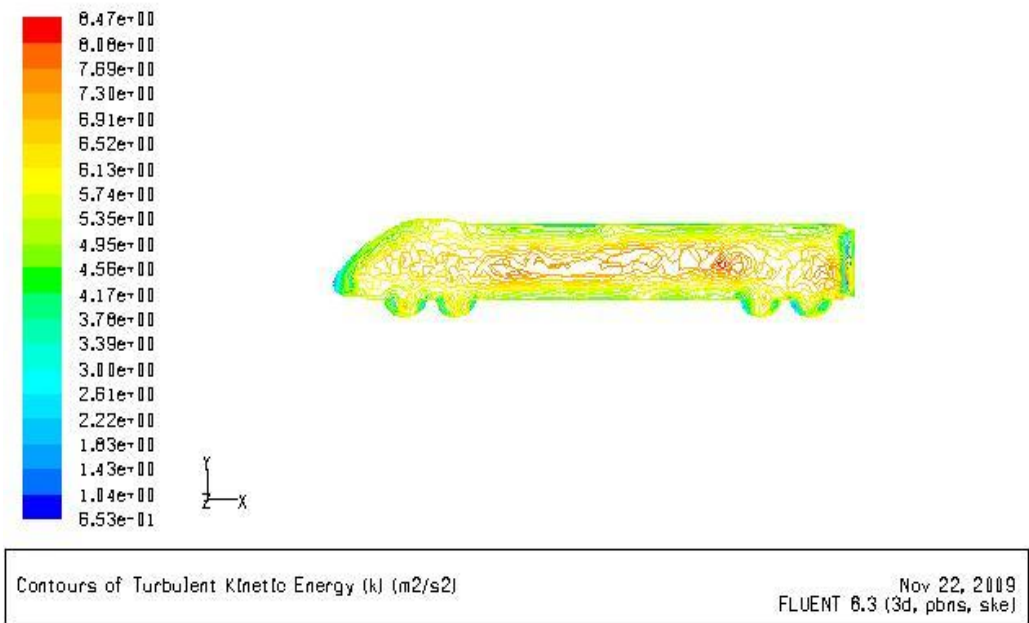
Figure 4.5 Turbulence Airflow as train speed is 50 m/s
