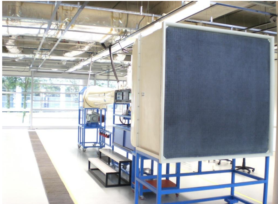
Figure 3.7(b) Wind tunnel equipment (rear view)
