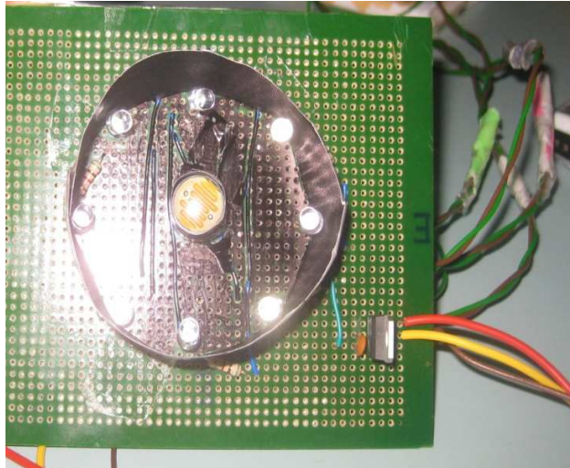
Figure 19 Color sensor built based on schematics
