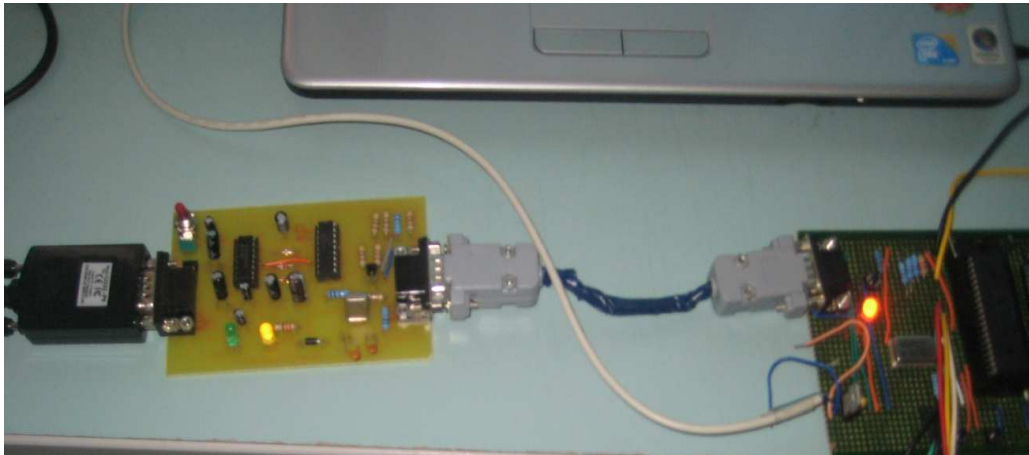
Figure 15 WISP628 programmer and microcontroller with LCD board on the left
