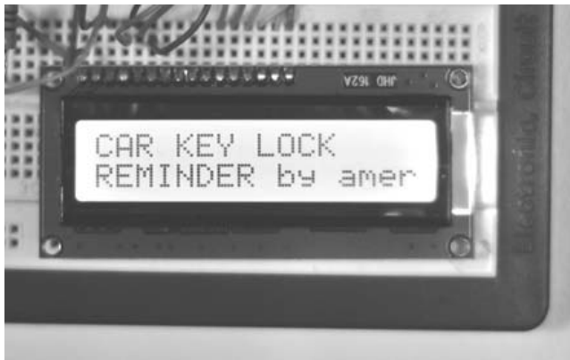
Figure 21 :LCD display 16x2 JHD1602A
