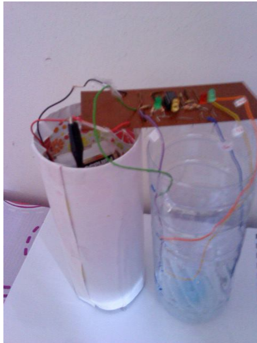
Figure 9: Water Level Circuit When Tank Is Empty
