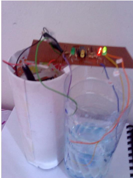
Figure 11: Water Level Circuit When Tank Is Half
