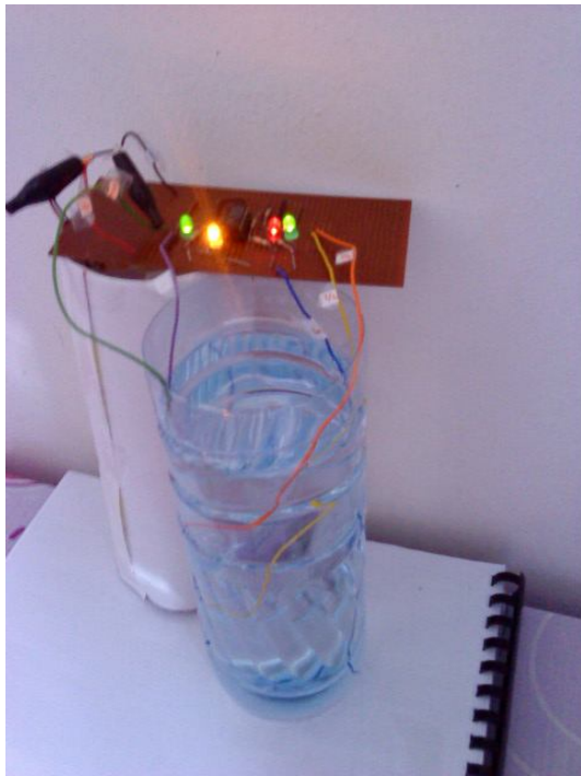
Figure 13: Water Level Circuit When Tank Is Full
