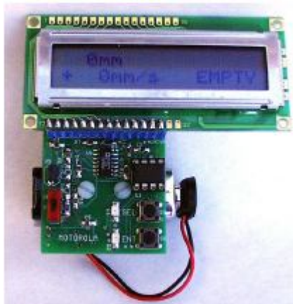
Figure 5: Water Level Reference Design Featuring a Pressure Sensor
