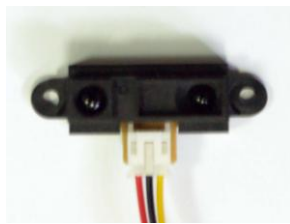
Figure 4.7 SHARP IR sensor (GP2Y0A21YK)
