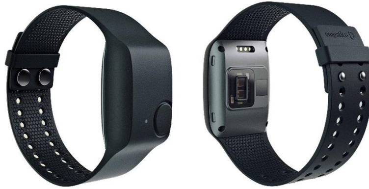
Figure 10 The Empatica E4 wristband allows the real-time measurement of EDA, blood volume pulse or skin temperature among other features.
