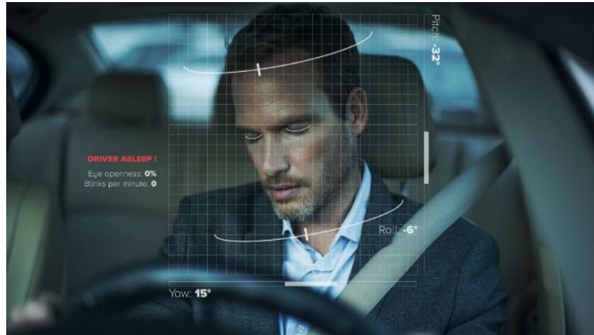
Figure 7 Example of a current DSM system from Cipia Technologies for the detection of driver drowsiness using eye-tracking and head positioning parameters.
