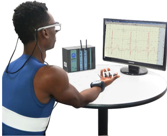
Figure 14 Biopac MP160 base station and wearable remote Bio-Nomadix amplifiers attached to the wrist with EDA sensors. Source: www.biopac.com
