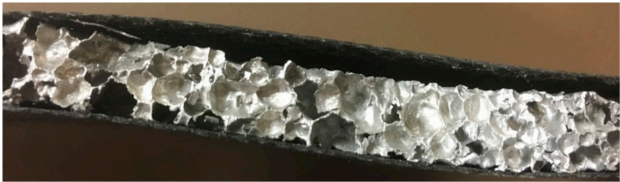
Figure 1. De-bonded AFS specimen subject to quasi-static load.
