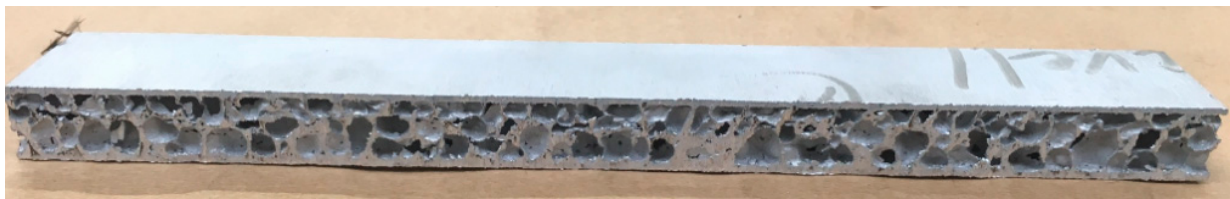
Figure 2. AFSS panel for this work.
