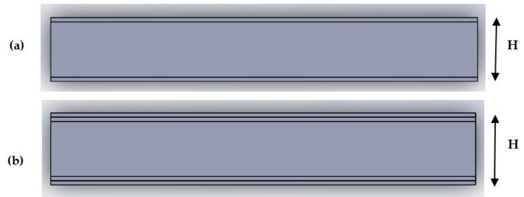
Figure 4. (a) 150 mm long AFSS panel only; (b) AFSS laminated with four layers of CFRP.
