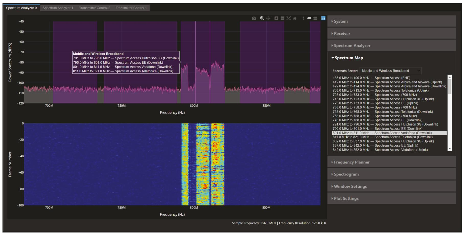
RFSoC-PYNQ is an open-source project from AMD that can make it easier to develop systems on RFSoC platforms. The StrathSDR team have developed an open-source spectrum analyser using RFSoC-PYNQ that can be deployed on the RFSoC4x2. The spectrum analyser can be accessed from a web browser. You can see a screenshot of the analyser to the right.
