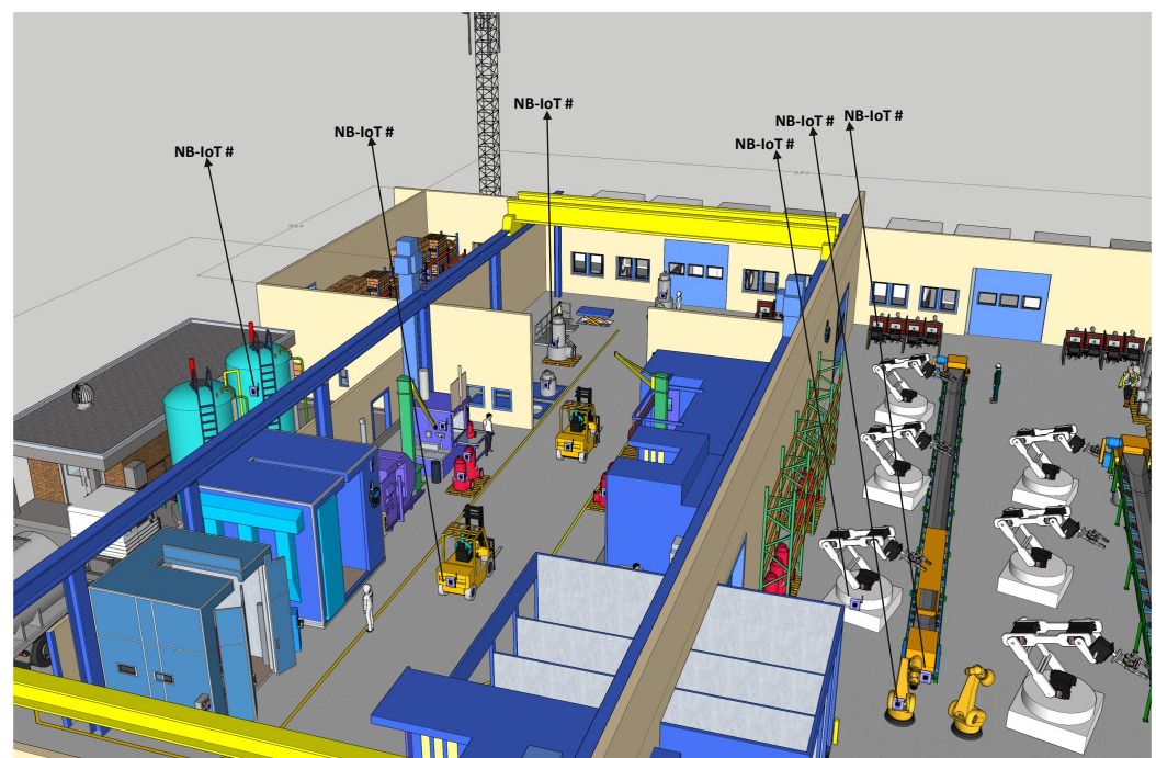
Figure 6. Diagram showing some of the positions of the NB-IoT terminals around the robotic arms, forklifts, and waste tanks.
