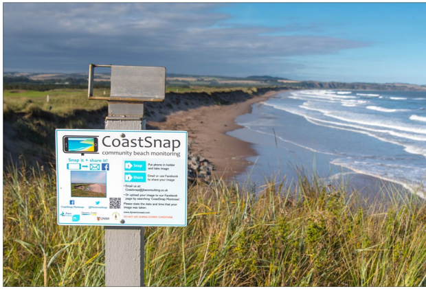
Fig. 2 CoastSnap beach monitoring, Montrose, Scotland. Members of the public are invited to monitor coastal erosion which is resulting in the retreat of the sand dune cordon, a natural form of coast protection, impinging on the adjacent golf course and increasing the risk of coastal flooding inland through several low-level corridors through the dunes. Strategic planning requires a shift from short-term engineering solutions at the coastal edge to dynamic, adaptational land management inland to provide space for relocation of assets to risk-free sites and to accommodate migration of the beach and dunes landward of their present position. This will require partnership and co-operative effort between all agencies, infrastructure providers, non-governmental organisations and businesses with a coastal remit or interest and supported by a funding stream (Rennie et al. 2021a, b) (photo: John Gordon)
