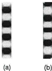
FIG. 2. Remanent state with (a) instantaneous and (b) gradual relaxation of the applied field.
