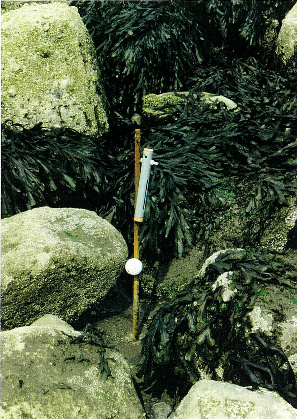
Figure 1.10. Maximum wave-force measuring equipment (low shore, Red Wharf Bay).
