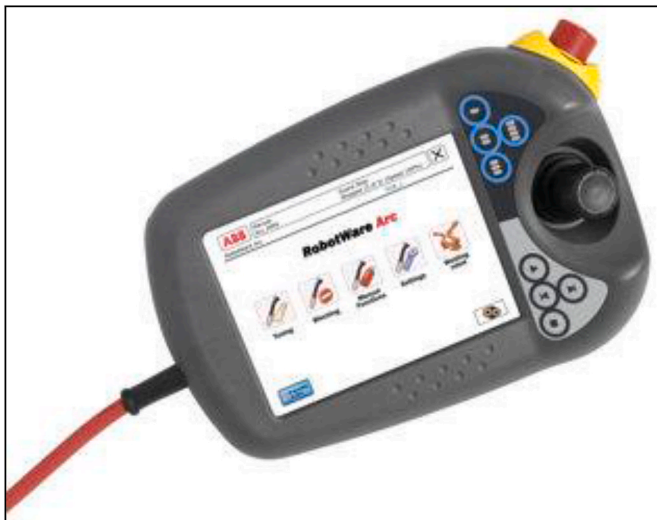
Fig. 1. An example of an RTP: The ABB IRC5 FlexPendant (Wernholt, 2007).
