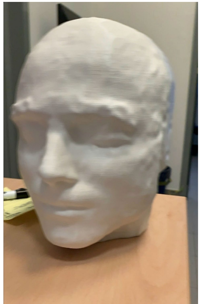
Fig. 6 The 3D-printed head phantom obtained from a structural MRI dataset, used to develop the anchorage procedure
