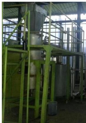
**Gambar 4.2** Gasifier Mini 50kg
