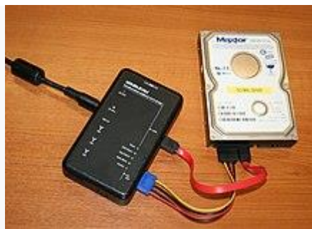
A portable Tableau write blocker attached to a Hard Drive
