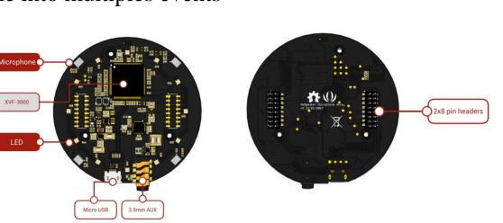
**Figure 6:** The top and bottom view of the ReSpeaker Mic Array v2.0 with labeled components
