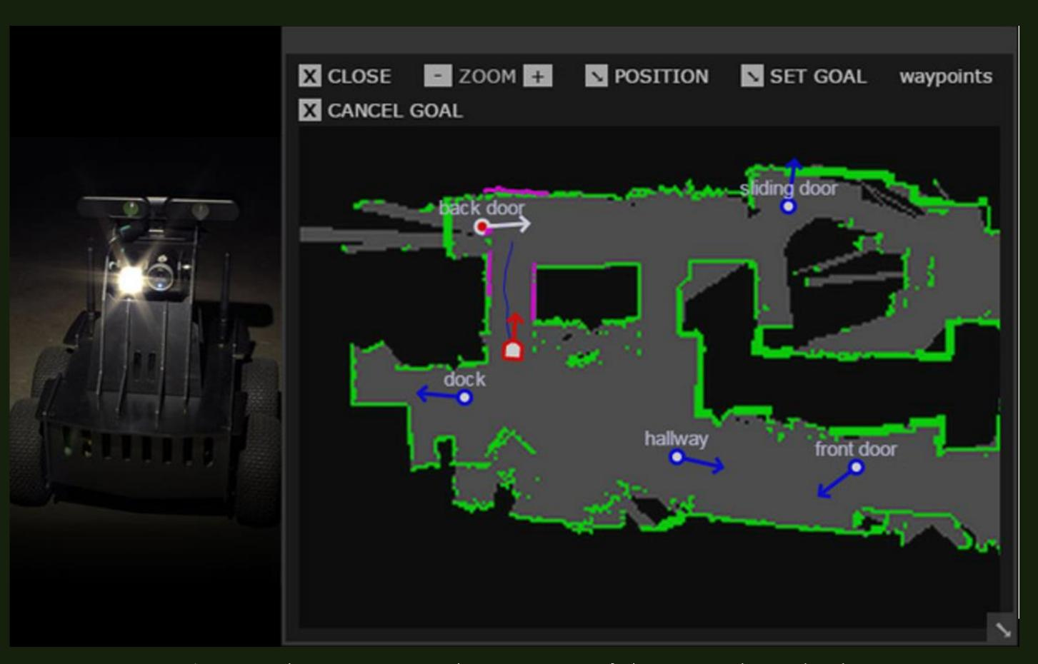
Figure 1: Oculus Prime navigator robot next to a map of a living space it has produced
